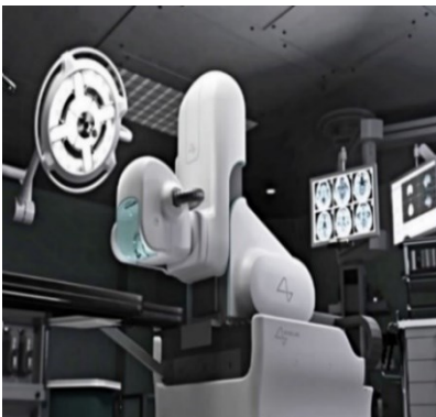
Figure 5. Neuralink robot that implants the threads.
